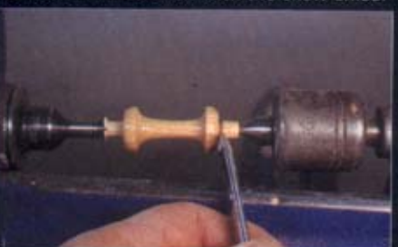
10 Part off the branch with the skew chisel
