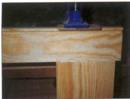
Any surplus Cascamite along the joint line can either be removed at the rubbery stage or sanded off when dry. Avoid removing with a wet cloth which spreads the glue
