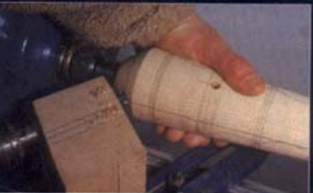
5 Cut the V-cuts with a skew chisel
