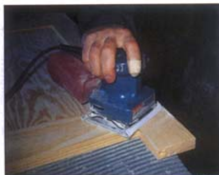
A palm sander is ideal for final smoothing, especially at the joints
