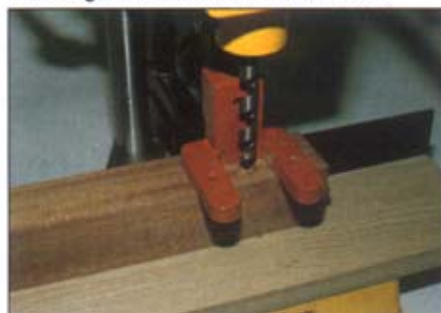
Boring with the hold-down shoe in use. The long bit is held in the main chuck
