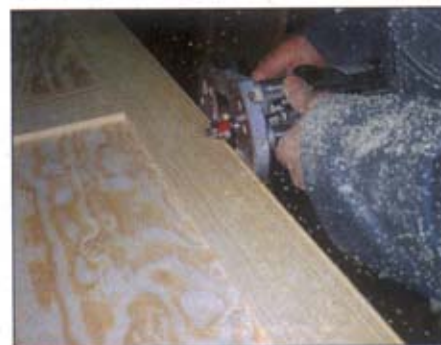
Cutting the 1/4"-diameter bead at the door sides with a bearing-guided beading cutter
