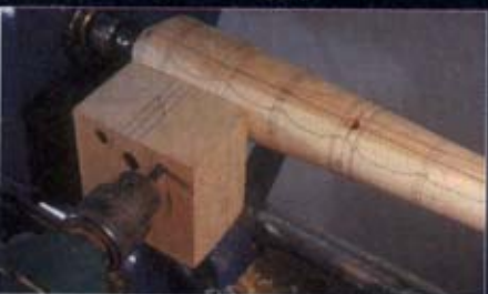
4 Drill the tripod leg holes
