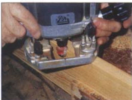
Using a bearing-guided beading cutter to form the 3/8" diameter bead on the outside of the frame
