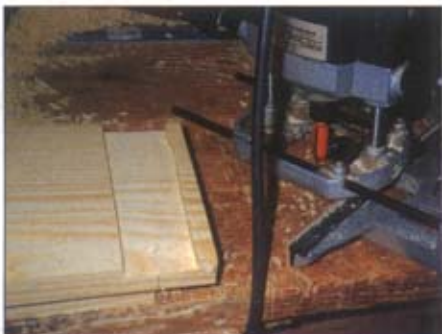
The tenons ready to be cut to length. Note the waste left on to guide the router
