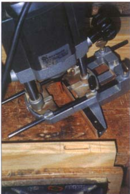
I cut the mortices using a router and a straight cutter guided by a fence
