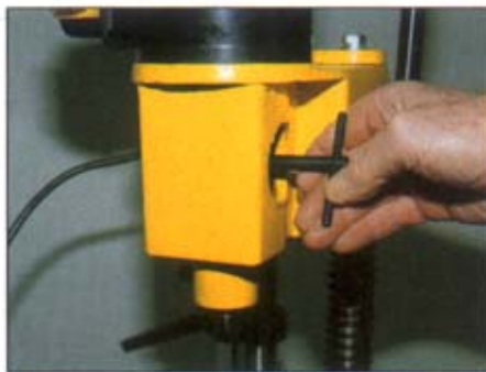
The chuck key is self ejecting so there's no fear of leaving it in the chuck
