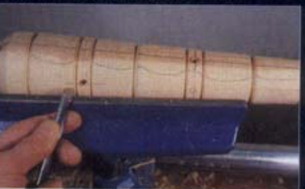
5 Cut the V-cuts with a skew chisel
