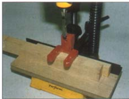
I added some packing behind the workpiece to set the chisel correctly
