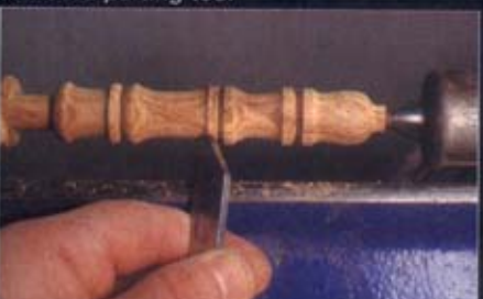
10 Part off the branch with the skew chisel
