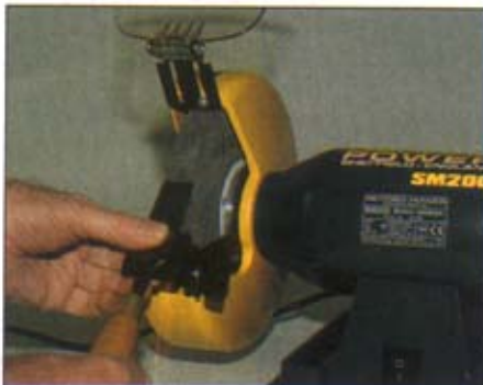
Grinding the chipped edge on a chisel
