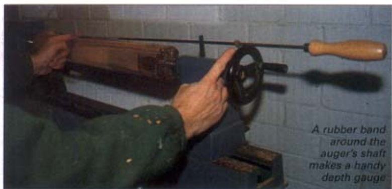
To counterbore, reduce the tailstock pressure, hold the blank stationary, and feed it carefully onto the revolving drive centre
