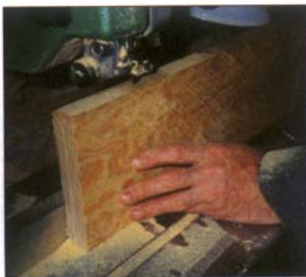
Resawing a 1" board to achieve the book-matching for the panels
