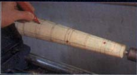
3 Drill out the dowel holes for the branches using a drilling jig
