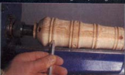
9 The same cut on the leg using the standard parting tool
